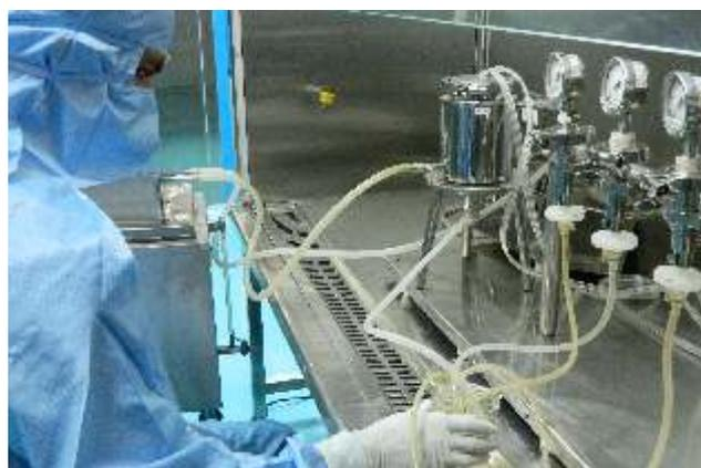
State of the art instrumentation and monitoring equipment coupled with flexible simulation jigs are used to achieve near perfect simulation of worst case process condition, an essential pre-requisite to filter validation with specific drug products.
