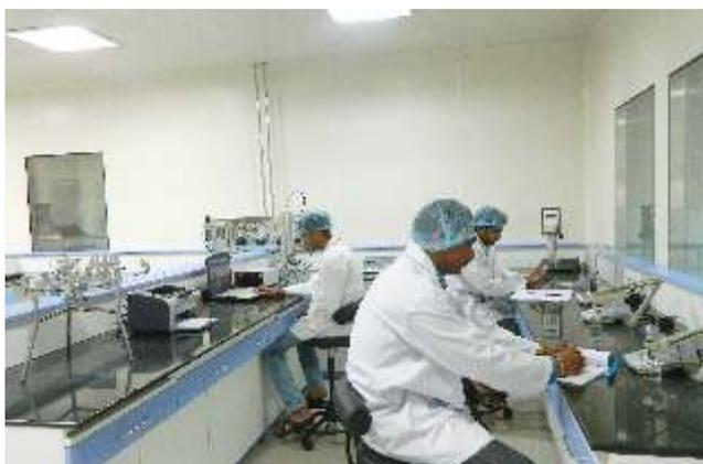
**mdi** Integrity test data generation lab is equipped with latest scientific equipment for filter integrity testing (FilterCheck) along with specially designed jigs and fixtures that incorporate simulation of critical parameters such as test temperature to ensure accuracy and reliability of data generated.
